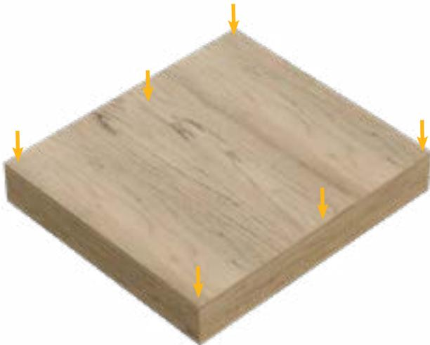
**Step 6:** Attach the surface to the saw platform by pre-drilling holes and joining with wood screws. Remember that the back brace is offset towards the front, so account for that when drilling in the back screw.
