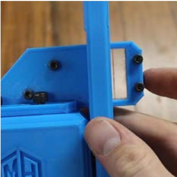
**Step 18:** Visually align the red marker line with the edge of the flip stop. Fine-tune this alignment with a scrap piece of wood by making a cut, measuring, and adjusting the sliding gauge on the stop block until it is correct, then tighten down. Finally, secure to workbench using the T-Track bolts.
