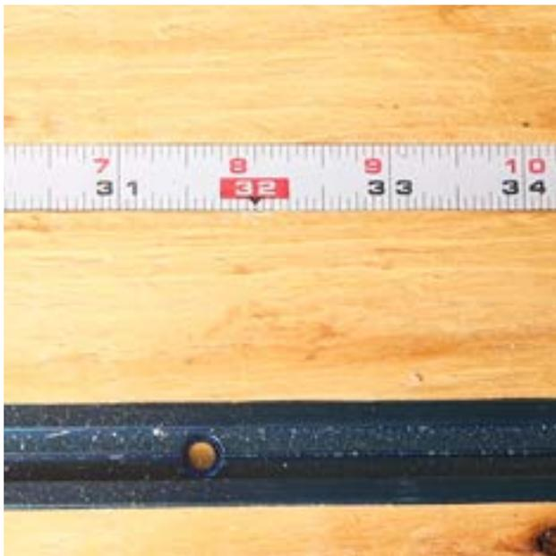
**Step 12:** Align the metal measuring tape with the line you marked out in **Step 11**, and remove the backing on the tape to permanently mount it into the shallow groove. I used a line of super glue as well, since the sticky backing on anything always seems to fail after a bit of use.
