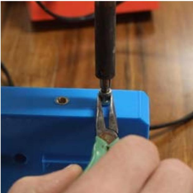
**Step 14:** Insert M5 heat-set inserts into the holes on the side of the stop block using a soldering iron. If you don't have heat set-inserts, an M6 bolt directly into the 3d printed part should work as well, though the holding power won't be the same.
