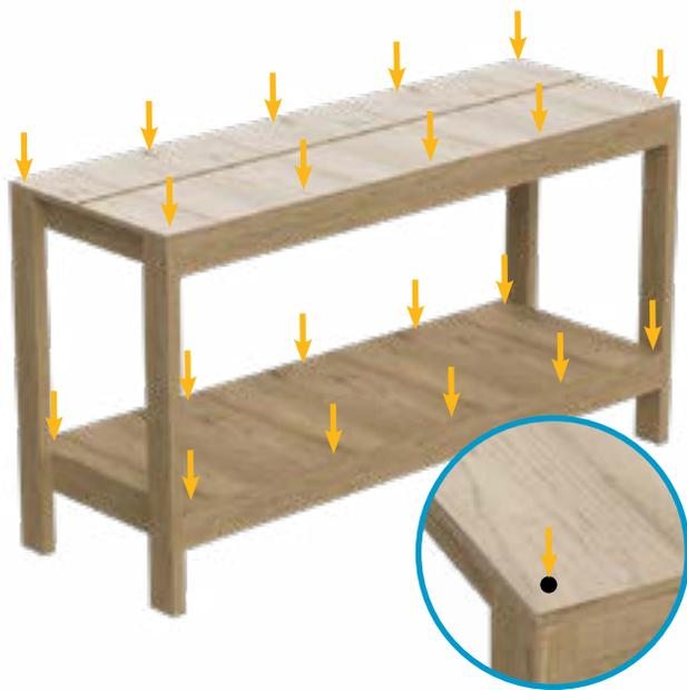
**Step 4:** After cutting the plywood down to size, attach each section to the frame by pre-drilling and mounting with wood screws. It is important to pre-drill here so the resulting work surface is flush and doesn't have screw heads protruding from it. Aim for the studs underneath, and avoid placing screws in the path of the T-Track, as you will need to route a track for that later. Repeat this process for the opposite side of the workbench.
