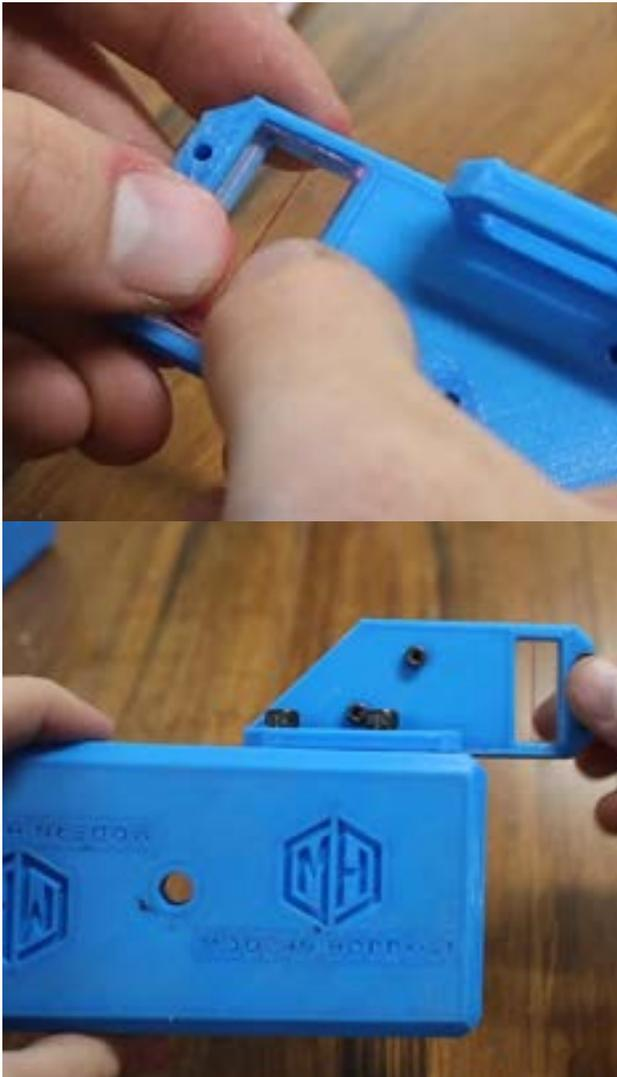
**Step 16:** Finish by assembling the line marking guide with M3 bolts, and repeat for the opposite stop block if necessary. Attach to the main body of the stop block with M5 bolts (if you used the heat-set inserts) and M6 bolts if you didn't.
